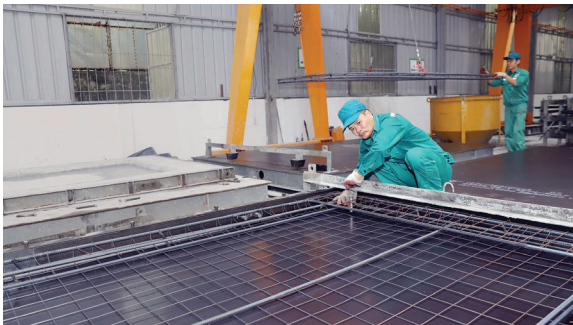
2. Laying reinforcement into mold
